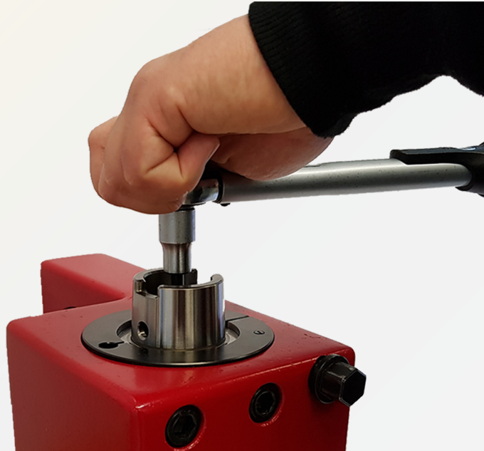
Fig. 11: Tighten clamping nut with torque wrench
