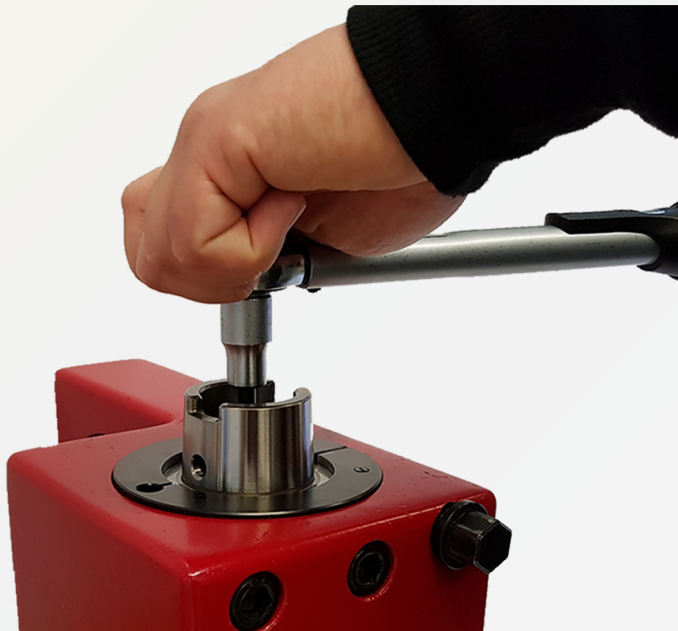
Fig. 7: Tighten clamping sleeve with torque wrench
