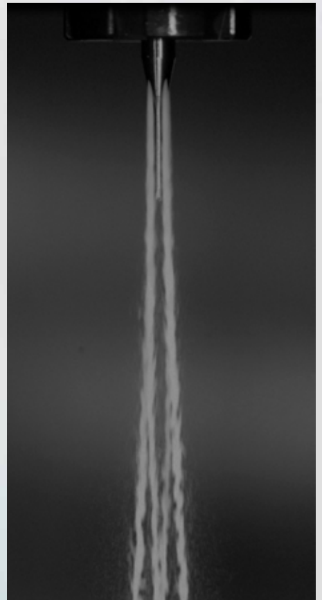
Internal cooling with 80 bar with S=24,000 rev./min
