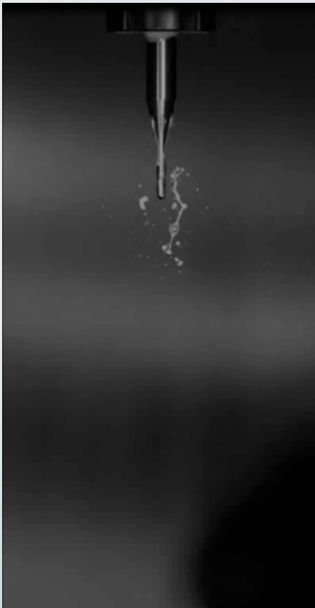
Switching on GuhroJet internal cooling
