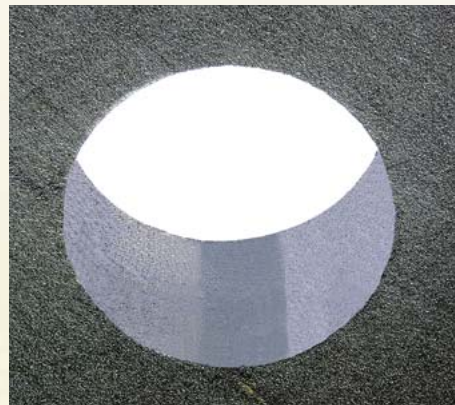
unidirectional CFRP hole D=6.35 mm
