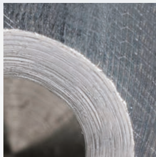
Countersinking with standard countersink
